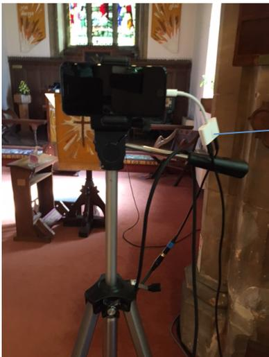
Loop wires around tripod handle to take weight and prevent plug from working loose
