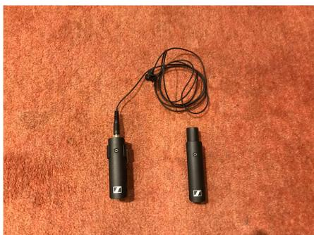
5. Holding the units close to each other press the switch on each unit until the green light momentarily flash and then show continuous green light (this should only take a few moments). The two units are now linked.
